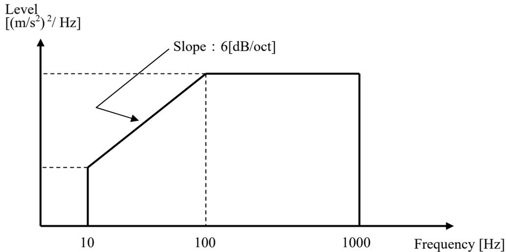
The PSD is specified to 10  $[(m/s^2)rms]$  having the shape as in the above between 10 [Hz] and 1000 [Hz].
