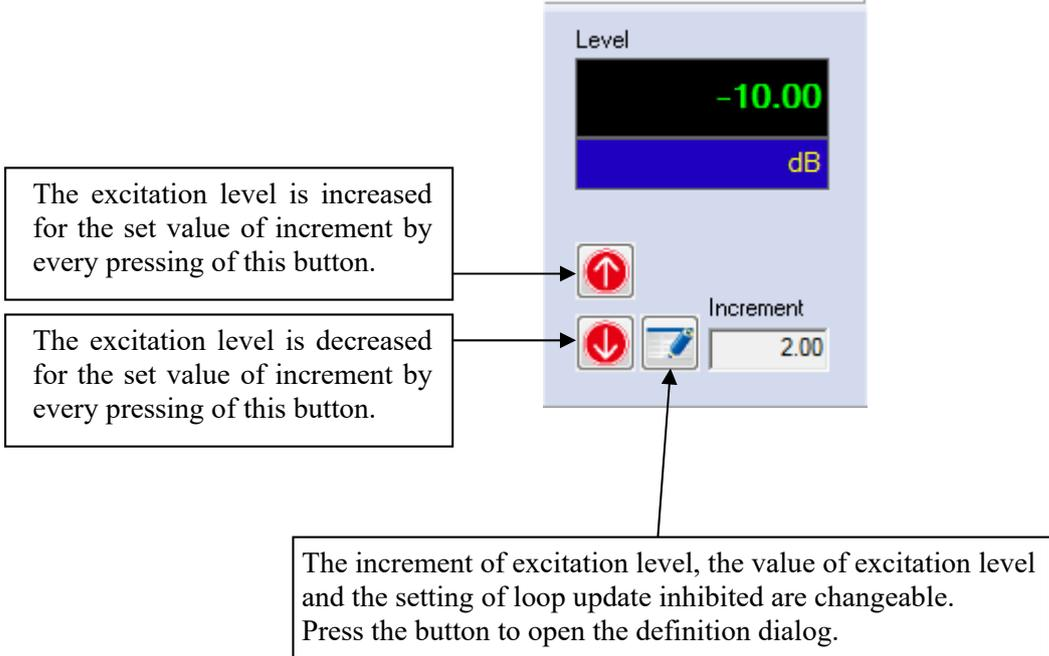
The excitation level is increased for the set value of increment by every pressing of this button.
