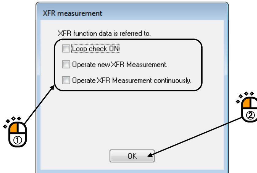
The phases of XFR Measurement is composed by Loop Check and XFR Measurement. Loop Check is needed to be executed for operating XFR Measurement. Four selections are provided in this item ;
