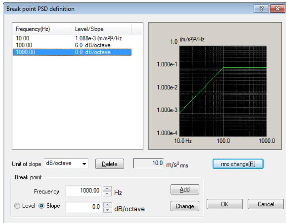
Break point PSD data definition is independent from the frequency resolution  $\Delta f$ . If the
