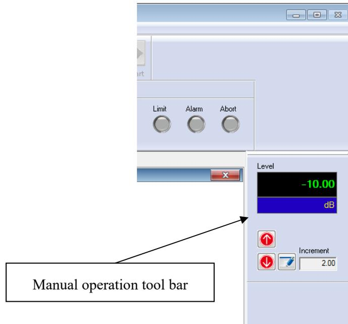
If the manual operation tool bar is not displayed, select [Display] in the menu bar and click [Manual operation tool bar]. Manual operation tool bar appears.
