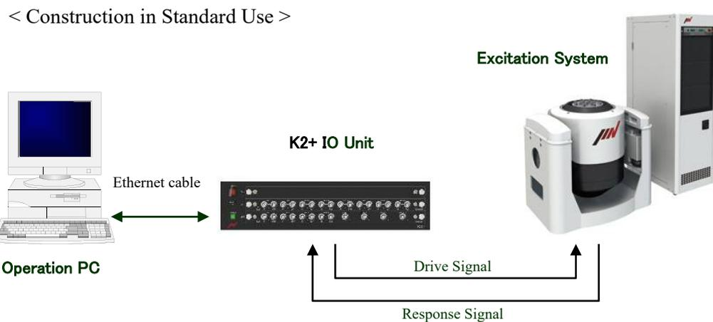
This manual provides instructions that you must observe to ensure safe and proper handling of the vibration control system. Before using this system, please read this instruction manual carefully to understand the contents thoroughly.
