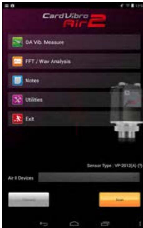
Touch "Scan" in the lower right corner of the main menu. Turn on the Air2 and make sure the red LED indicator is blinking.
