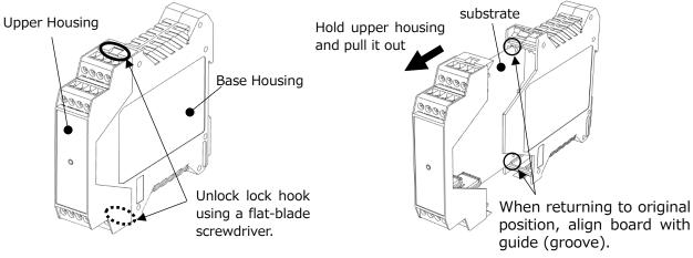
Fig.7-1 Pulling out upper housing
