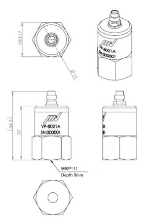
Outer Dimension of VP-8021A (Unit: mm)
