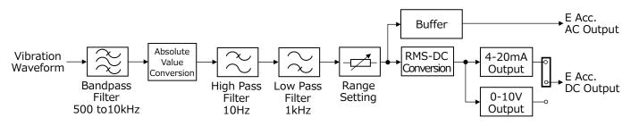
Fig.13-3 Block Diagram of E acceleration
