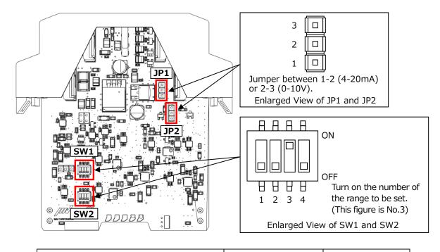
(4) Change measurement range and DC output according to Fig.7-2 below.
