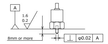
Fig.4-2 Processing of the accelerometer mounting surface
