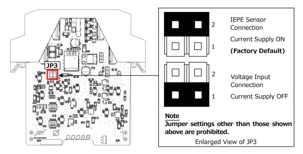
Fig.A-2 Drive Current Supply Setting
