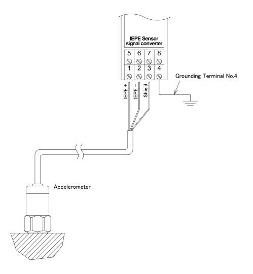
Fig.A-1 Wiring when the Accelerometer is not grounded
