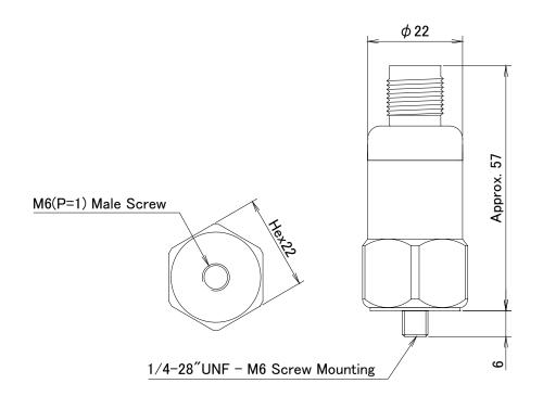
Outer Dimensions of the VP-1001005406 (Unit: mm)
