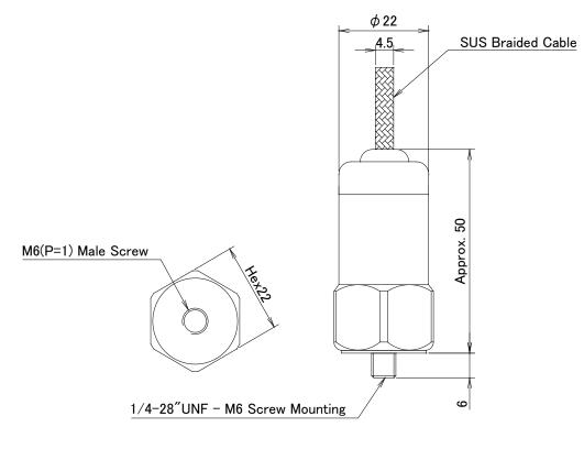
Outer Dimensions of the VP-1001000206 (Unit: mm)
