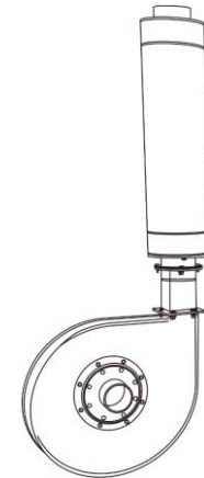
Blower a: W 1,160 mm b: H 2,405 mm c: D 787mm
