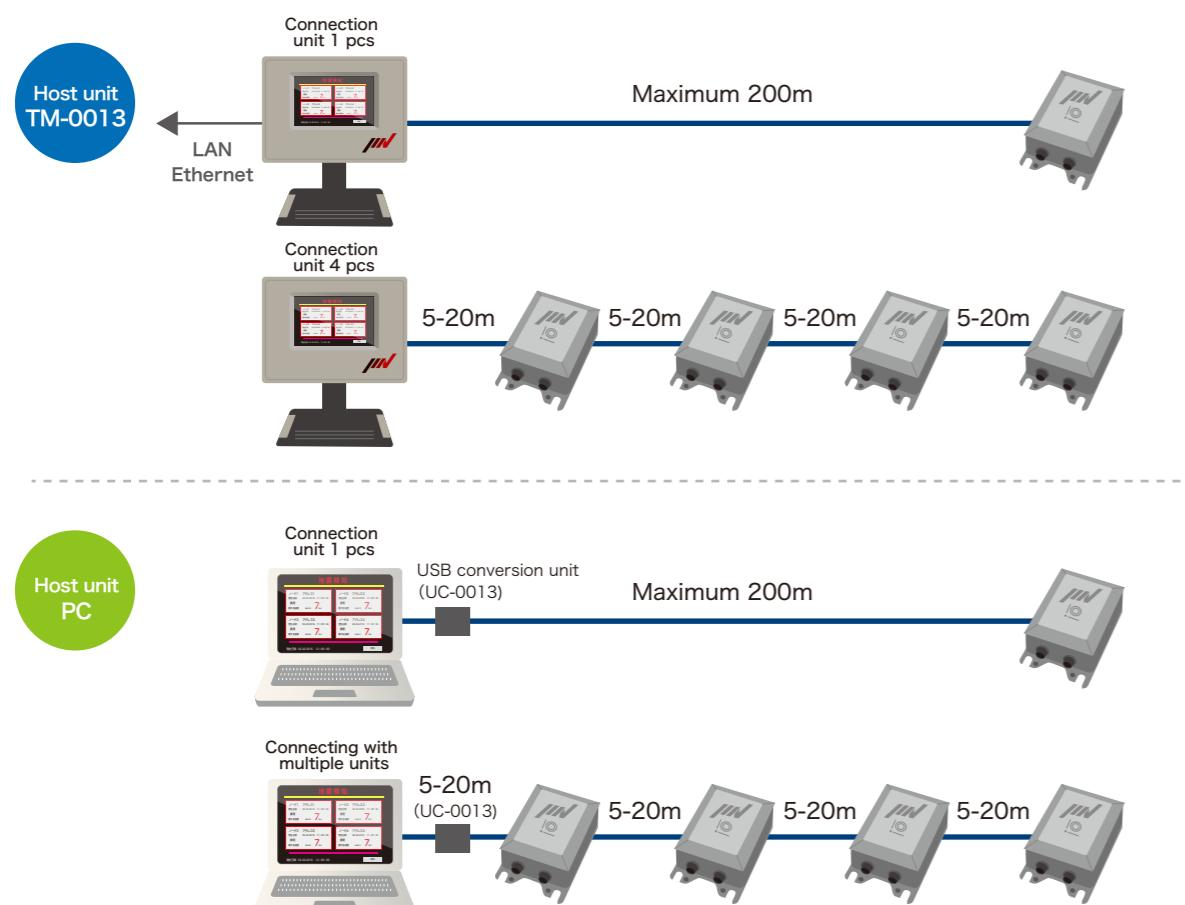
By using Power Junction Box RP-0013, technically speaking, there is no limitation for cable length. Please contact us for length and system quantity. When the number of unit increase, it may limit some part of functions.
