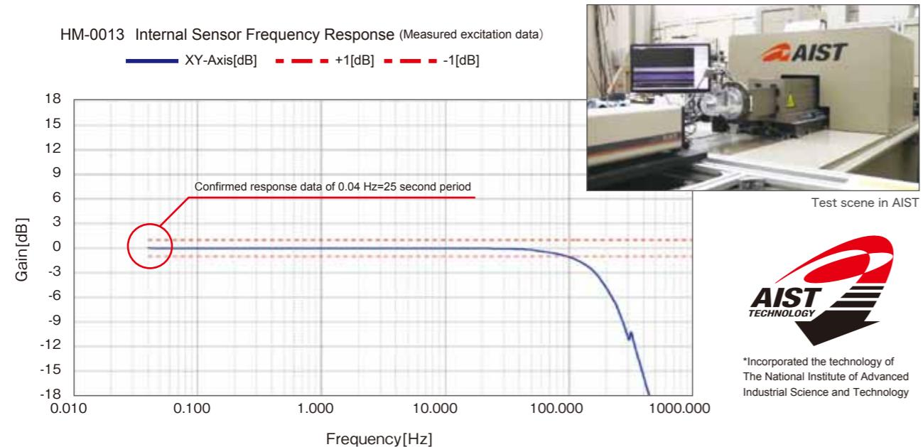
Operation verification at low frequency 0.04 by AIST\* has proven that HM-0013 can detect the long-ground motion accurately.
